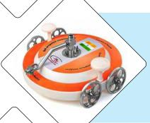
In contrast to the cavitation jet, which is unmatched for cleaning complicated structures, the main tool for cleaning large areas —for example, the hull of a ship — is the self-propelled cleaning device (Self-propelled Cleaning Device, SCD). It has a wide working area and moves at high speed on cleaning surfaces; it allows you to clean even large areas to a high quality in a very short time.
